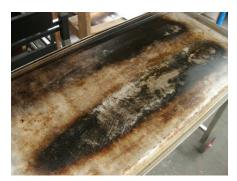
This plate is made of 3CR12 which is a grade of stainless steel suited to this purpose as it is the "best" conductor of heat, although not as good a conductor as mild steel. This 3CR12 plate is magnetic. It is composed of 12 to 18% chrome, no nickel and a low carbon content, and is termed "ferritic". It has a fair to good corrosion resistance.
