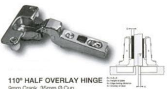
9mm Crank. 35mm Ø Cup. 10mm Plastic Dowels at 52mm C.
